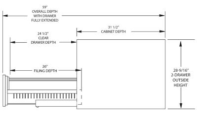
2 Hour Fire, Impact and Explosion Rating The Schwab Series 5000 vertical file has met Underwriters' Laboratories stringent requirements for the classification of 'Record Protection Equipment.' This includes a test for fire-resistance in external temperatures exceeding 1850°F for two hours, a 2000°F explosion hazard test as well as a test to withstand the impact of a 30 ft. drop.
